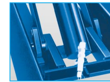
OIL FLOW CUT-OFF VALVE against hydraulic breakage
